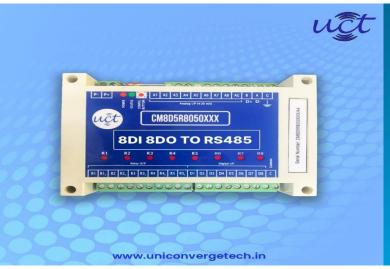
8 Digital Input 8 Digital Output to RS485 converter module converts the 8 digital input and 8 digital output data to RS485.
