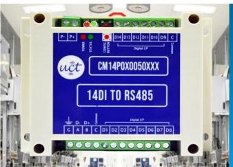
The 14-Digital Input to RS485 Modules accept 14 Digital Inputs from various industrial sources
